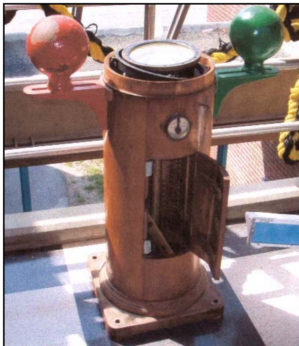
Figure 3 Magnetic Compass in its binnacle (Photo by C. Weeks). Magnets go in the open door. The red and green iron spheres are Quadrantal Correctors. The magnets and Quadrantal Correctors correct for deviation.
